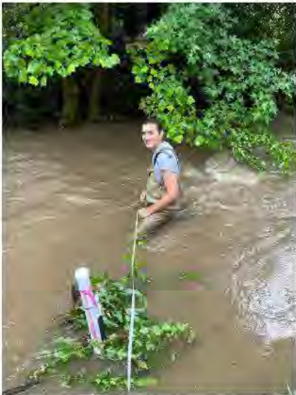
Discharge Measurements at 1/2 Bankfull
